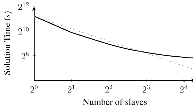
Figure 3.3: Solution time against the number of slave processes showing actual (solid) and ideal (dashed) scaling rates.
